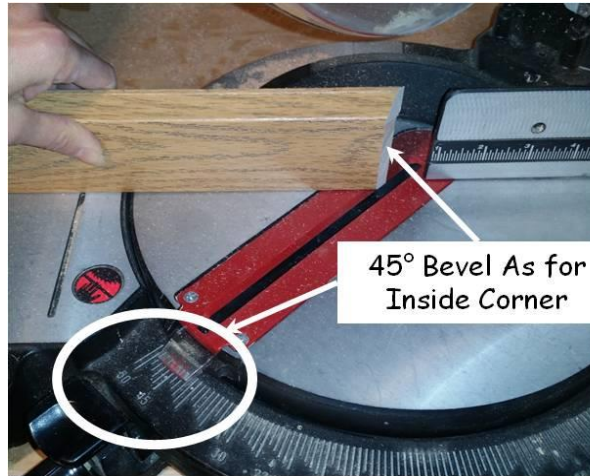
Figure 19-1. Base Trim Bevel Cut.
